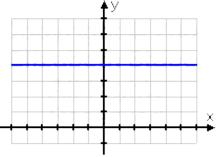
In the example here, every point on this line has a y-coordinate of 4. So some examples of points on the line would be (1, 4), (0, 4), (10, 4), (3, 4), (5, 4), (2, 4), (4, 4) and so on. The list is limitless.
